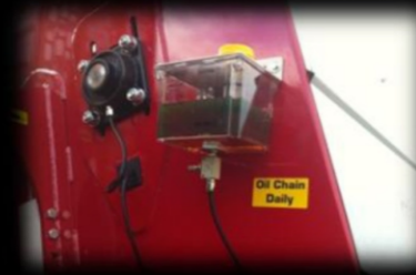
Elevator Chain Oilers
