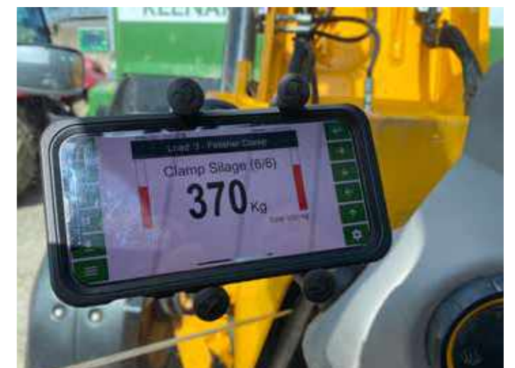
The InTouch app enables Rhodri to use his smartphone as a remote version of the machine's control panel.
