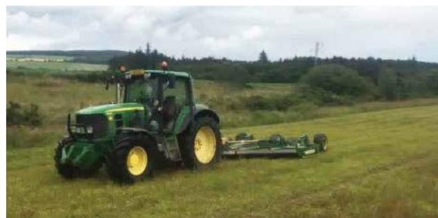
Four gearbox drive line, each with an independent slip clutch for each cutter assembly to minimise drive line shock in rough conditions. This drive layout allows the wings to operate from -20° up to transport positions (90°).
